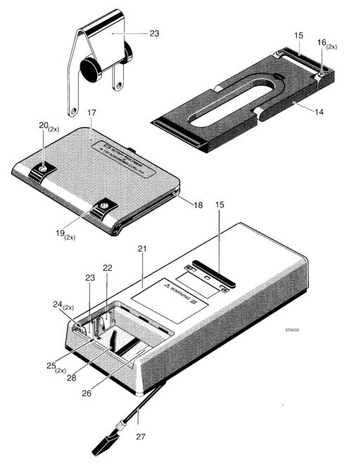
Figure 7.10 Replacing parts in battery compartment
